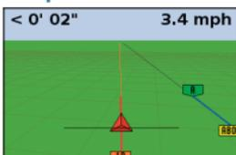
By default, the view automatically switches to the perspective view when you enter a field. To set the view so it switches when you engage an autosteering system or for manual view control, in Advanced mode select **Configuration / System / Display / View**.
